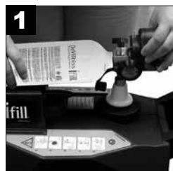
Put bottle assembly on personal oxygen station.
