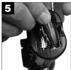
Install batteries if necessary (observe polarity).
