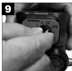
When you are finished using the iFill oxygen cylinder, turn the rotary selector to the "OFF" position.
