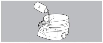
Fill the humidifier up to the "max." mark with cold distilled water.
