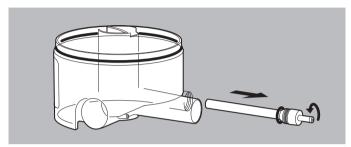
2. Unscrew the heater rod from the lower part of the housing.
