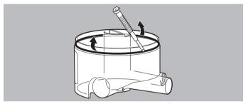
2. Use a screwdriver to remove the seal carefully without damaging the groove.
