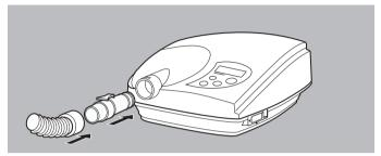
1. Plug adapter onto device outlet port.
