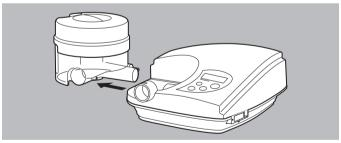
1. Push the humidifier sideways out of its locator.
