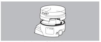
7. Screw together the parts of the housing.
