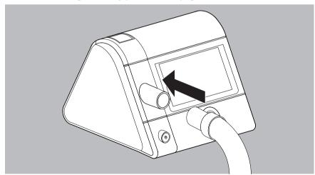
2. Push breathing tube onto the device outlet port.
