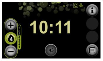
The humidifier levels 1-7 are available. The setting suitable for you depends on the room temperature and humidity. Humidifier level 4 is the standard setting. If you have dry airways in the morning, heating output is set too low. If condensation has formed in the breathing tube in the morning, heating output is set too high.
