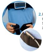
2. Put the abdomen strap around the abdomen as shown. The pressure sensor is to be inside the belt.
