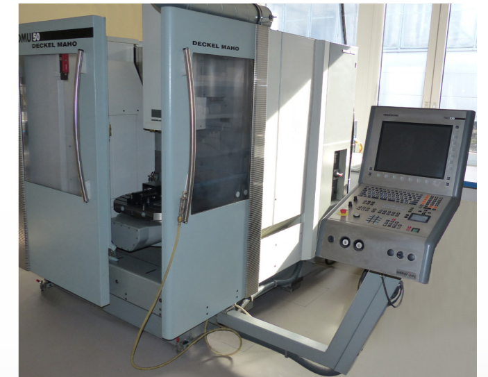
Milling machine for the production of aluminum forms
